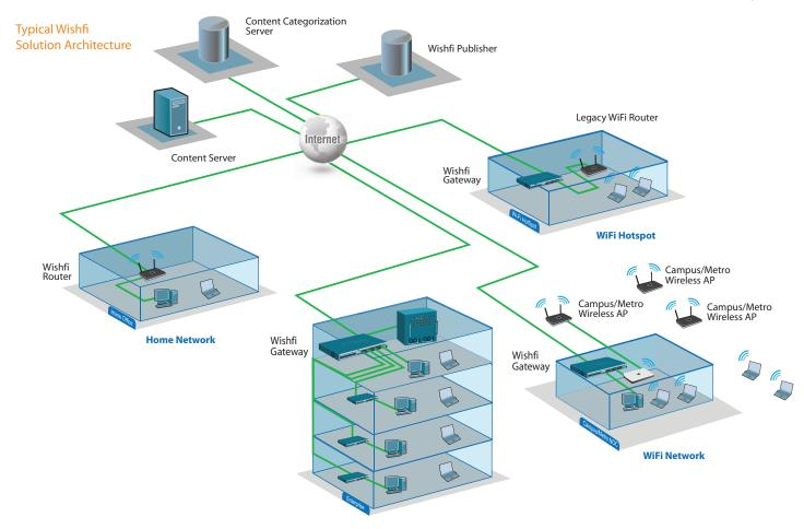
Typical Wishfi deployments include: Wishfi servers running in the customer or D-Link's Network Operations Center, a variety of remote web content or advertising servers providing content, WiFi hotspots with targeted services for visitors, and Wishfi-enabled routers or gateways at remote locations (or VPN access to remote sites with legacy routers).
